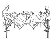
3. Each partner should then grasp the bottom of the middle frame section (cross beams) where it forms diamond. Lift slightly and slowly walk backward until the frame is fully extended. Be careful not to pinch your finger and not pull backward too hard as this may result in the bending of cross beams.
