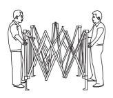
1. Stand frame upright. Starting at the corners, with partner standing on the opposite side, grasp the two outer legs, slightly lift the frame off the ground and step backward, stopping at full arms' length.
