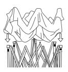
2. Place the fabric top over the frame but do not fix it. You may always place the fabric top later till the frame fully opened if it's too heavy to you to do the set up with fabric top.
